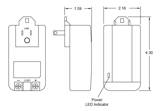
Description Plug-in Class II Regulated Power Supply with LED power
