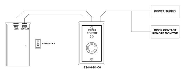
**Pushbutton Unit** used for Failsafe Control of Secured Doors
